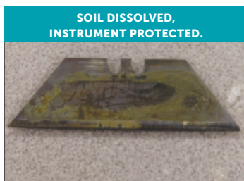
Razor blades after 15-hour soak in ProEZ foam show corrosion arrested and soils dissolved.
