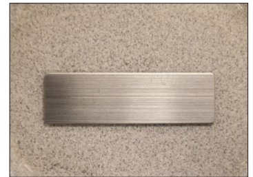
TOSI™ washer test coupon, sprayed with ProEZ foam and held 72 hours.
