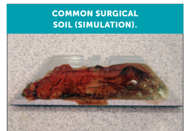
Razor blades with animal blood surrogate applied show early corrosion after one hour.
